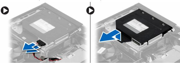
5. Flex the optical-drive bracket and then lift the optical drive from the bracket
