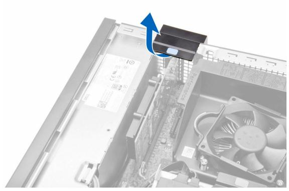
**6.** Pull the release lever away from the expansion card until you release the securing tab from the dent in the card. Then, ease the card up and out of its connector and remove it from the computer.
