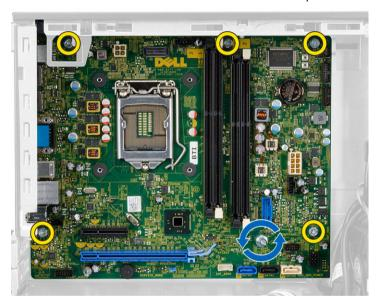
6. Remove the system board from the chassis.
