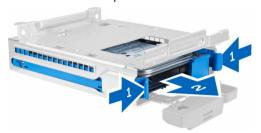
4. Flex the hard-drive bracket and remove the hard drive from the bracket.
