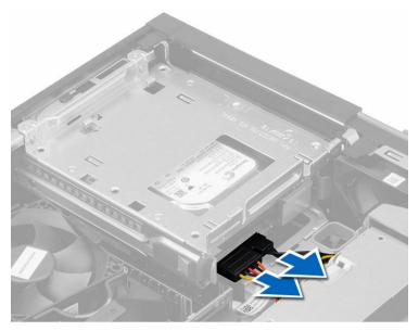
4. Slide the blue drive-cage handle toward unlock position and lift the hard drive cage from the computer.
