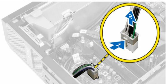
4. Disconnect the 4-pin power cables from the system board.
