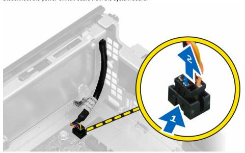
**4.** Press the clips on both side of the power switch to release it from the chassis and remove the power switch along with its cable from the computer.
