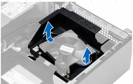
4. Disconnect the fan cable from the system board. Loosen the captive screws, lift the heat sink assembly and then remove it from the computer.
