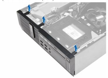
**4.** Rotate the bezel away from the computer to release the hooks on the opposite edge of the bezel from the chassis. Then, lift the chassis and remove the front bezel from the computer.
