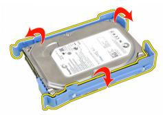
Remove the screws that secure the mini hard drive to the hard-drive bracket and remove the hard drive from its bracket.
