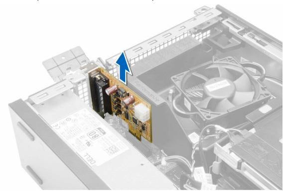
$\textbf{5.} \hspace{0.5cm} \textbf{Rotate the release tab on the card-retention latch upward.} \\$
