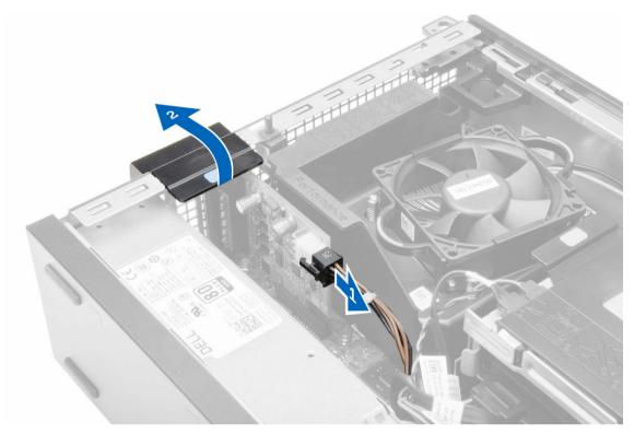
**4.** Ease the card up from its connector and remove it from the computer.
